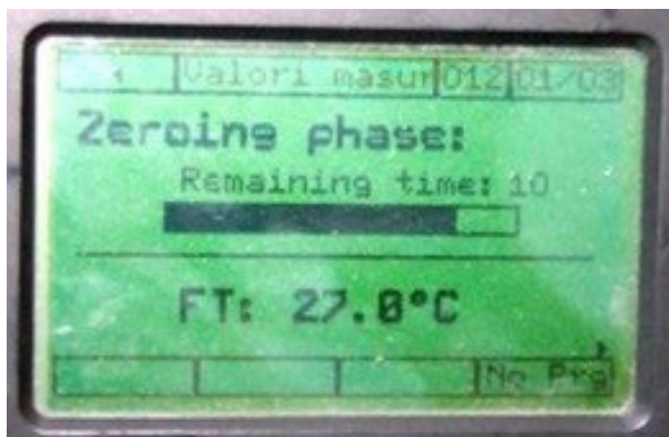
Figure 3. Zero calibration procedure of the Testo 350 M/XL analyzer.
